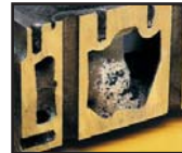
Severe corrosion can occur when additives that protect the cooling system have been depleted.
