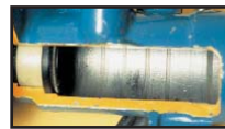
Grooves are worn into the soft metal of the spool valve housing by hardened seals. Metallic debris from such wear accumulates in the fluid causing premature component failure!
